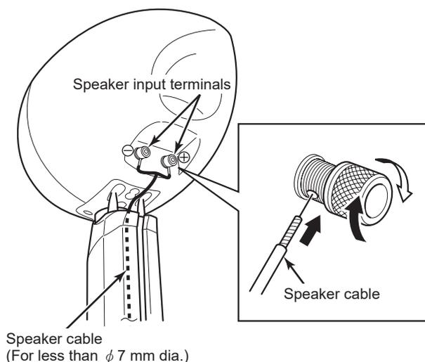
Speaker cable (For less than  $\phi$  7 mm dia.)
