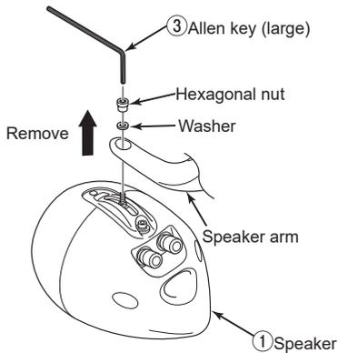
**4** Remove the hexagonal nut and washer which are securing the speaker unit and the speaker arm.
