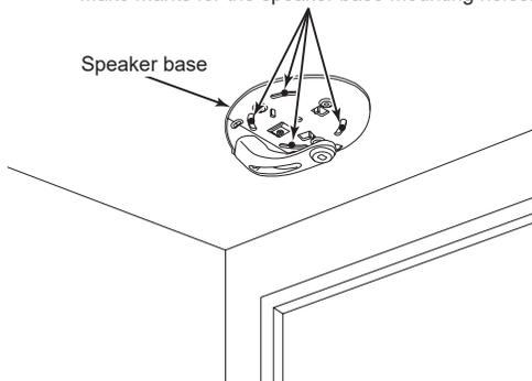
**1** Use the speaker base to determine the installation position for the speaker on the indoor ceiling, and then use tape or similar to attach the speaker base to the ceiling.
