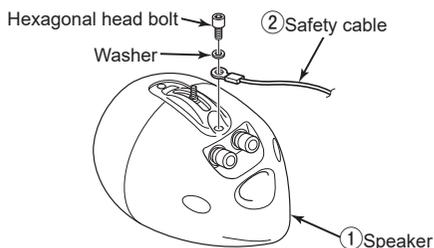
**6** Fix the safety cable to the speaker unit.
